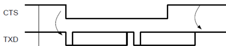
Figure 30-23: Transmitter Operation Behavior When Hardware Handshake is Enabled
