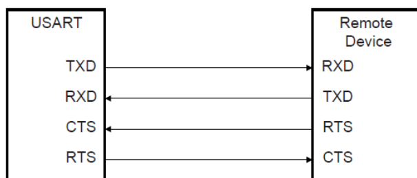
Figure 30-21: Hardware Handshake with Remote Devices
